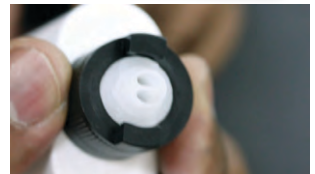
Attach nut and turn until tight
